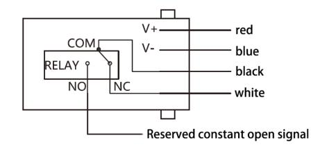
Note: The difinition of the output line is based on the actual product label. The above image indicates the status of each wire after power in aplied. One reserved normaly open signal wire is used for the lower limit disconnection and uper limit connection.
